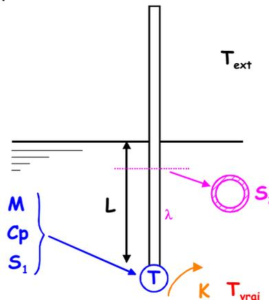
$$\text{D'où, } MCp \frac{dT}{dt} = KS_1(T_{\text{vrai}} - T) + \frac{\lambda S_2}{L}(T_{\text{ext}} - T),$$
